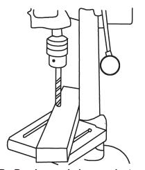
Figure D: Bracing workpiece against column
